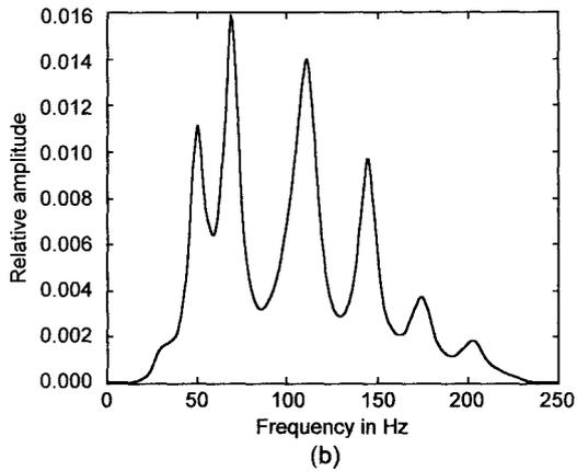
**Figure 5.** (a) The FFT spectrum of the EMG signal sampled at 500 Hz. (b) The AR model spectrum of the same EMG segment with 20 coefficients calculated using the covariance method.
