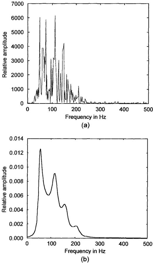
**Figure 3.** (a) Spectrum of Surface EMG segment calculated using FFT. (b) AR model spectrum for the same segment using 20 coefficients calculated using the covariance method.
