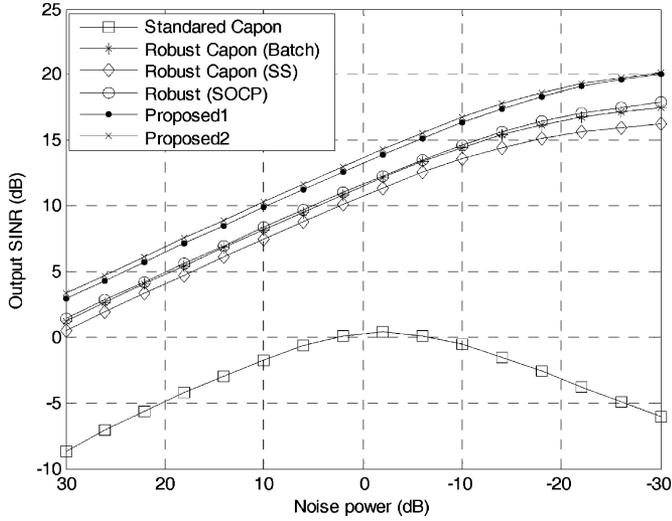
Fig. 8. Output SINR versus noise power with  $0.03\pi$  mismatch.
