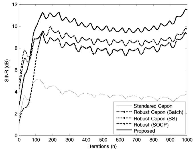
Fig. 15. Output SINR versus snapshot for non-stationary moving scenario.
