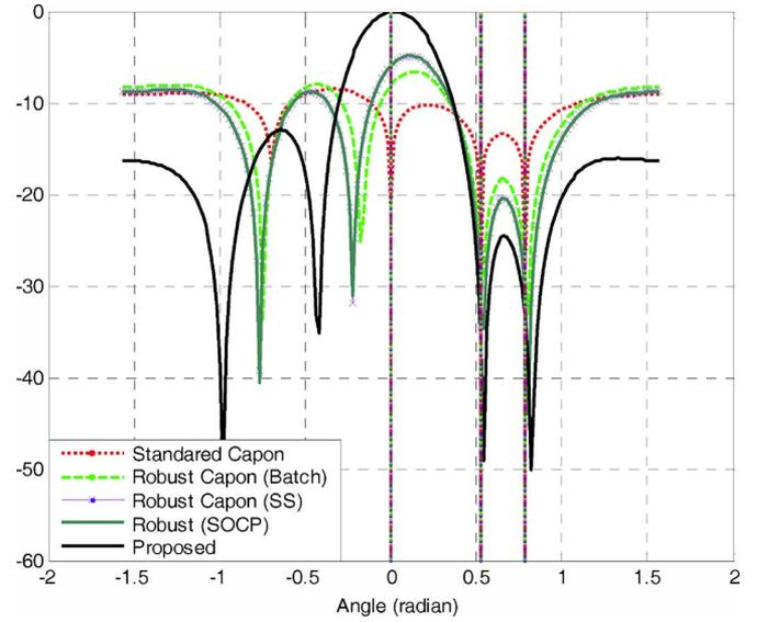
Fig. 6. Steady state beampatterns for the first scenario.
