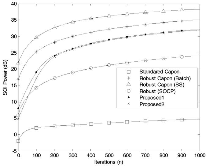
Fig. 4. SOI power versus snapshot for first scenario.
