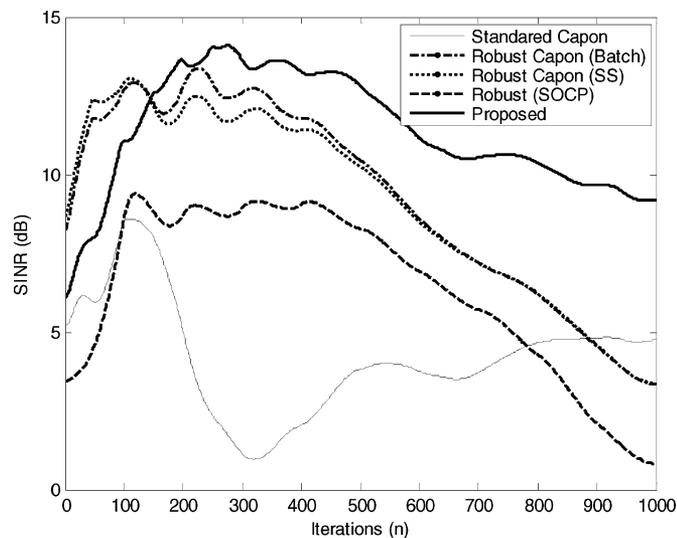
Fig. 14. Output SINR for coherent stationary moving sub-scenario.
