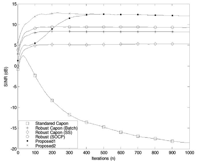
Fig. 7. Output SINR versus snapshot for the second scenario.
