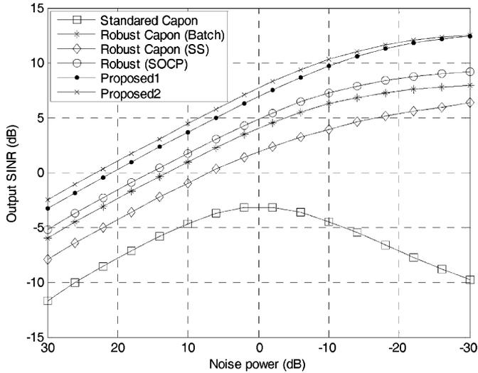
Fig. 9. Output SINR versus noise power with  $0.06\pi$  mismatch.
